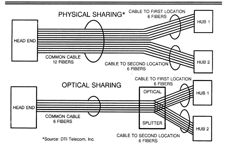
than only one as in traditional configurations. Thus, a major advantage of a fiber upgrade is the reduction in the number of amplifiers in cascade, thereby increasing channel capacity, enhancing signal quality and reducing maintenance costs; additional benefits include system redundancy, improved reliability, increased bandwidth channeling for future upstream signaling, and the potential for private (addressable) and two-way point-to-point communications.
