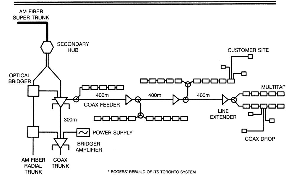
distribution system, which accounts for 70% of total plant miles, is capable of transmitting at 1000MHz. Although transmission will initially be at 550MHz, installing capacity for 1000MHz will avoid the cost of rebuilding when transmission capability expands. Optical bridgers, interfacing fiber and coax, will extend the fiber network past the secondary hubs to the coaxial cable network which feeds about 200 homes.
