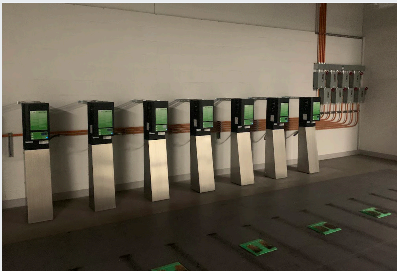
Charging stations for the Cleveland Clinic's self-charging, materials-handling autonomous robots
