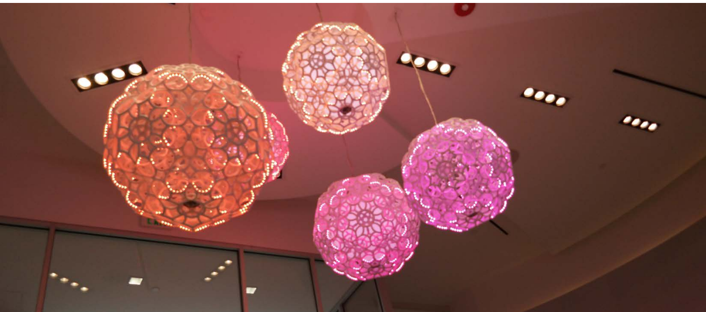
Chandeliers in the lobby at CATA. There are five pieces made up of 160 polycarbonate parts that were printed on their machines. 5,000 LEDs light up the globes, each with their own IP address. Normally, the parts would have taken a year of total print time but CATA was able to do it in just 2 ½ months running 12 of their machines 24 hours a day.
