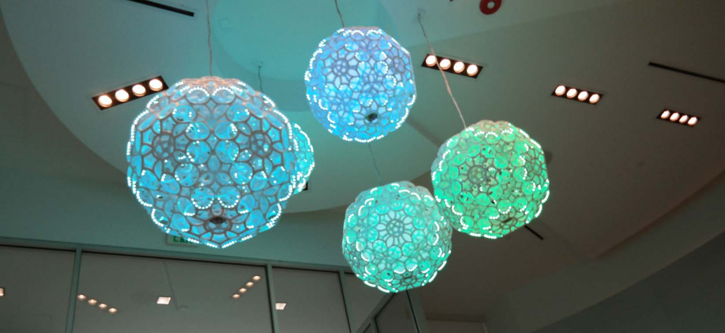
Chandeliers in the lobby at CATA. There are five pieces made up of 160 polycarbonate parts that were printed on their machines. 5,000 LEDs light up the globes, each with their own IP address. Normally, the parts would have taken a year of total print time but CATA was able to do it in just 2 ½ months running 12 of their machines 24 hours a day.
