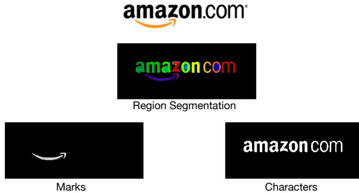
Figure 2: Examples of the segmentation process, using Amazon’s logo as an example. The original logo is at top. Beneath that is the segmented logo, where black identifies the background, and distinct regions are marked by different color regions. We then apply a template matching and filtering algorithm to identify which of these regions are characters (bottom-right), and assume the remainder are the marks (bottom-left).
